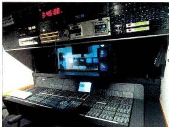
This Euphonix CS-2000 56-channel audio board is complemented by a digicart and surround-sound capability. Video monitor at center can display all setup and working menus, waveforms and selected metering. Each input channel features two direct stereo outputs and eight auxiliary outputs. (Photo courtesy of Lin Productions.)
