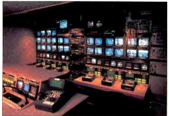
Slo-mo controllers are a must for trucks used in sports applications. Each controller can be patched for use with any of the tape machines located in the center of the monitor wall.
